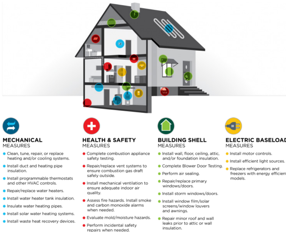
Graphic: Department of Energy, "Typical Weatherization Measures"
